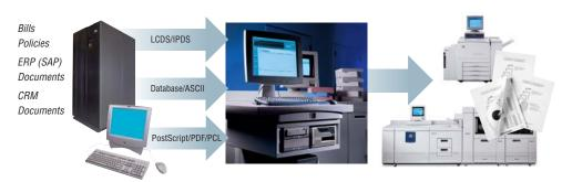
The DocuPrint® EPS allows you to effortlessly print applications from data center, copy/reproduction, and office environments. It supports Line Condition Data Stream (LCDS), Intelligent Printer Data Stream (IPDS) from the mainframe or network, PCL, Adobe PostScript® 3, PDF, and TIFF from the network.
